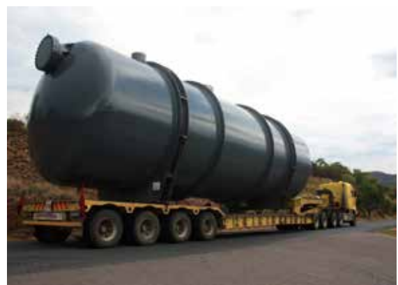
One of six 200 m 3 condensate tanks for Eskom Madupi Power Station manufactured by Pelindaba Enterprise
